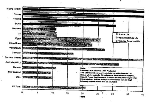
SPDC, Norway, Malaysia and Brunei cannot produce their currently booked gas reserves without significant increases in production rate compared with 2001. For illustration, production would need to increase by the following amounts in each case by 2008 – and hold constant thereafter - to ensure production of the booked within-licence reserves:
