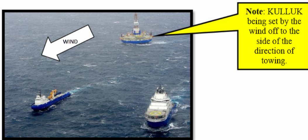
Figure 32: NANUQ on the left and AIVIQ on the right side of the photo with the KULLUK under tow in the distance (USCG Photo)
