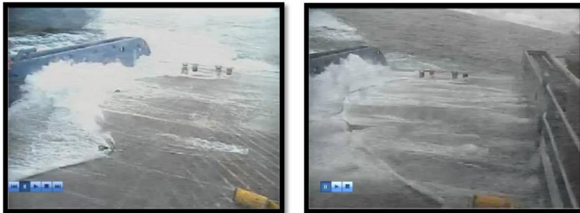
Figure 71: (left) Still from Port Forward CCTV showing seawater flowing over aft working deck and entering safety deck area at 14:39:09 on December 27. (right) Similar occurrence at 14:49:19 on December 27. (AIVIQ CCTV Provided by ECO)
