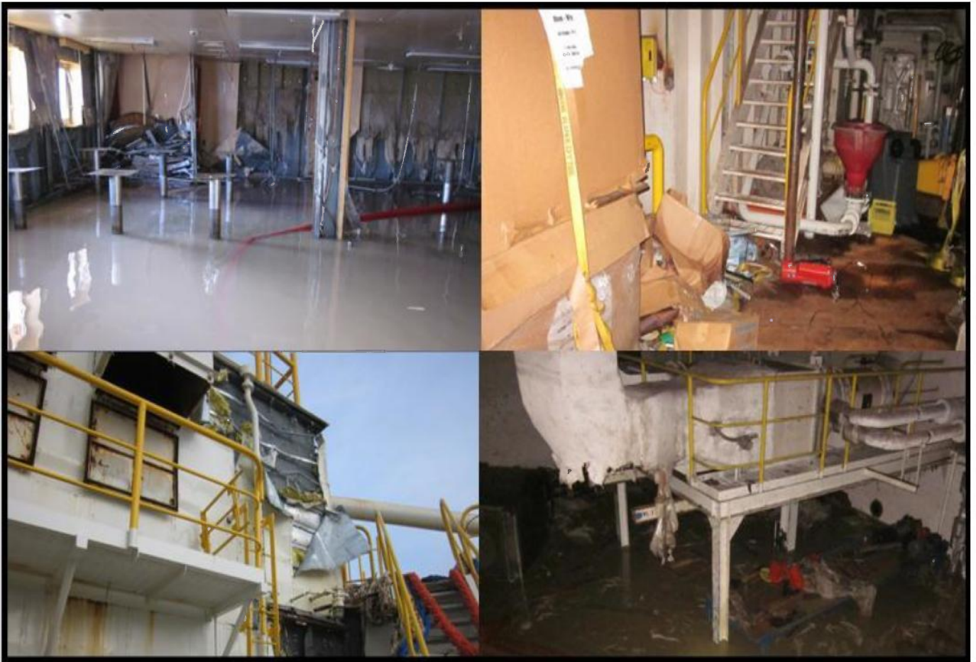
Figure 45: Composite photographs showing damage to topside areas of the KULLUK taken by USCG Inspectors after the grounding and prior to refloating. ( USCG Photos )
