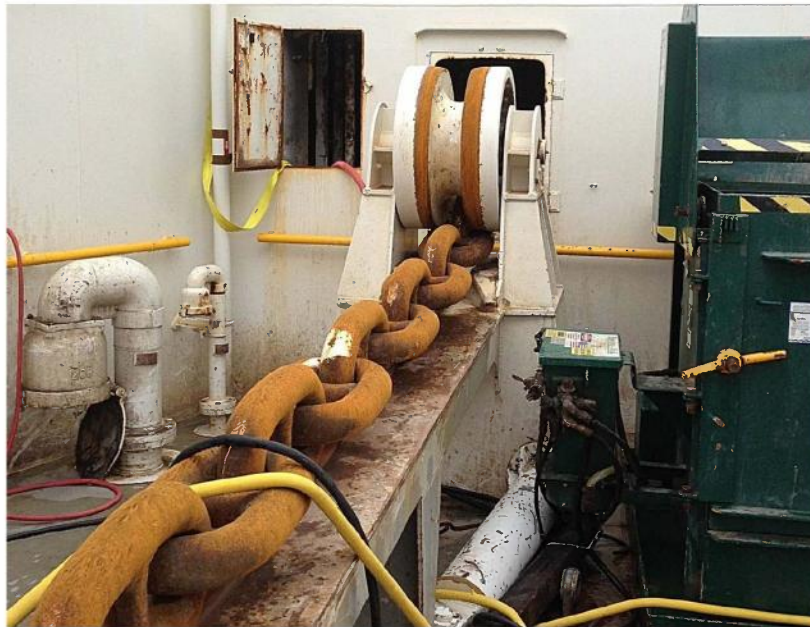
Figure 30: The anchor chain for the survival anchor leading out of the windlass room towards the hawsepipe. (Photo provided by Shell)
